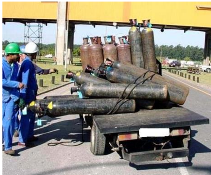
Unsecured cylinders or poorly secured cylinders will move and result in accidents.
